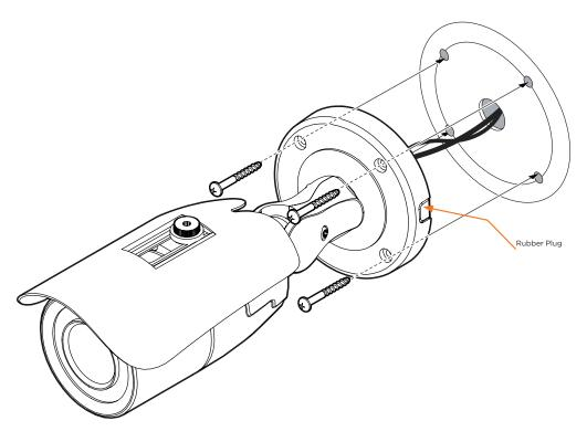
NOTE: Based on the installation environment, remove the rubber plug on the side of the camera's bracket and use the gap as a cable guide to prevent cables from getting caught between the camera and the mounting surface, which can cause damage to the cables and prevent the camera from mounting flush with the mounting surface.
