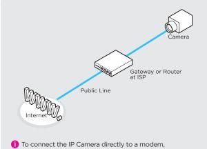
Io connect the IP Camera directly to a modem, power down and reset the modem. Leave the modem powered down until the IP camera's setup is completed and the IP camera has been connected to the modem. Then power on the modem, followed by the IP camera.
