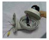
Insert the wires from the camera through the wall mount housing.
