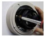
• Secure the lens with the two screws.
