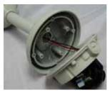
Slide the wires from the camera through the pendant mount.
