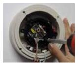
Secure the camera module to the surface mount with the four screws.
