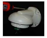
Use the mounting template to make pilot holes. Use the dry wall anchors and machine screws to attach the assembly to the wall.
