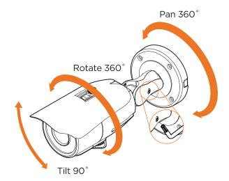
3. To adjust the camera's focus and zoom, remove the lens cover. Unlock the zoom and focus screws by rotating them counterclockwise. When done, tighten the screws and close the front case by rotating it clockwise.
