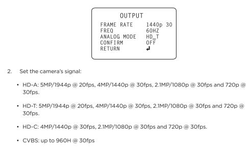
Change CONFIRM to ON and press the joystick to save the changes.
