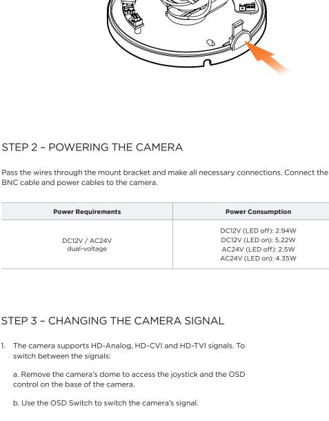
To switch the camera to HD-TVI mode, press the OSD joystick to the left for 5 seconds.
