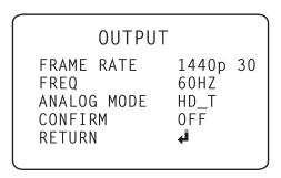
NOTE: To use your Star-Light Plus<sup>™</sup> 5MP cameras at a lower resolution, you must use a VMAX® A1 Plus™ DVR to access the camera's menu due to the cameras being set to 5MP as the default. A DVR that does not support 5MP resolution may recognize the camera, but will not deliver a picture
