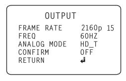
NOTE: To use your Star-Light Plus™ 4K cameras at a lower resolution, you must use a VMAX® A1 4K DVR to access the camera's menu due to the cameras being set to 4K as the default. A DVR that does not support 4K resolution may recognize the camera, but will not deliver a picture.
