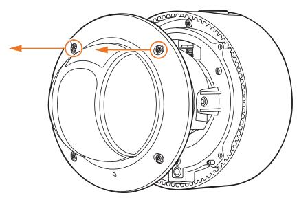
2 Using the screws included with the sun shield, assemble the camera's dome and sun shield cover following the diagram below. See the camera's QSG for more information.
