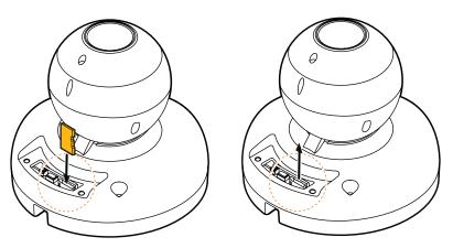
**NOTE:** Maximum SD Card size supported: Up to 1TB micro SD / FAT32. When inserting the SD card into the card slot, the SD card's contacts should be facing upward, as shown in the diagram.
